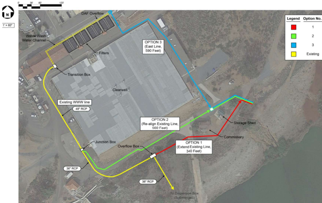
Figure 5.29 Backwash Realignment Alternatives
