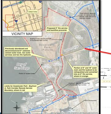
Port of San Diego would accept facilities "as-is" and would install 8-inch fire service (approx. 11 LF long) with backflow preventer
